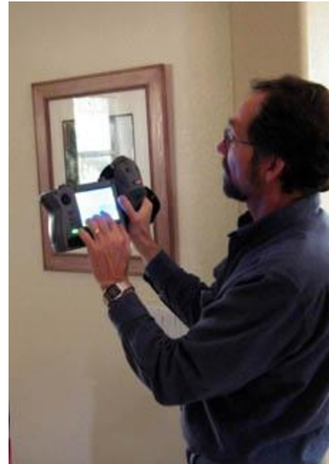
Wahl uses an infrared camera to detect areas of low energy-efficiency. Enterprise photo by Krissi Krob
